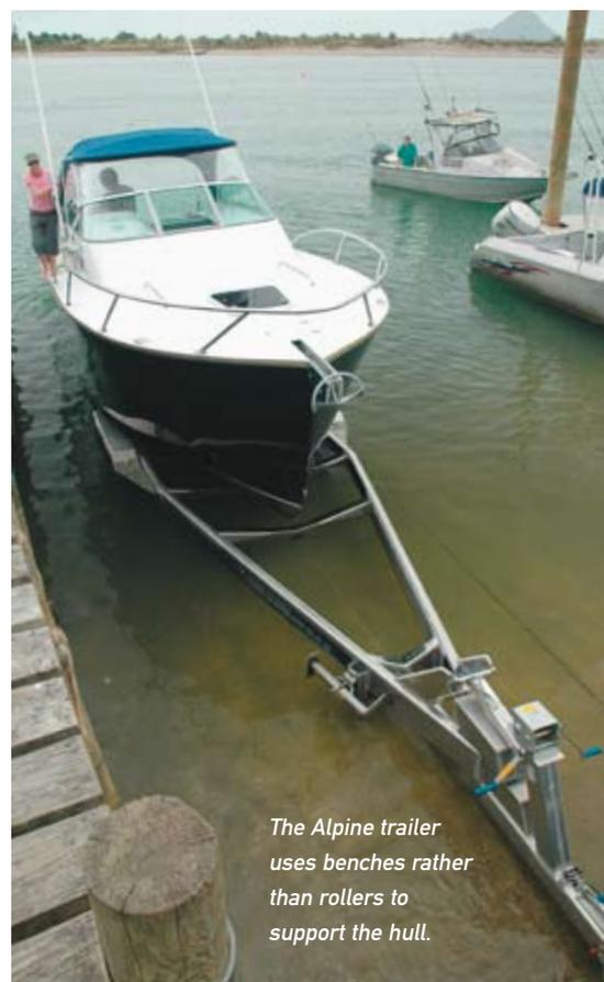
The Alpine trailer uses benches rather than rollers to support the hull.
