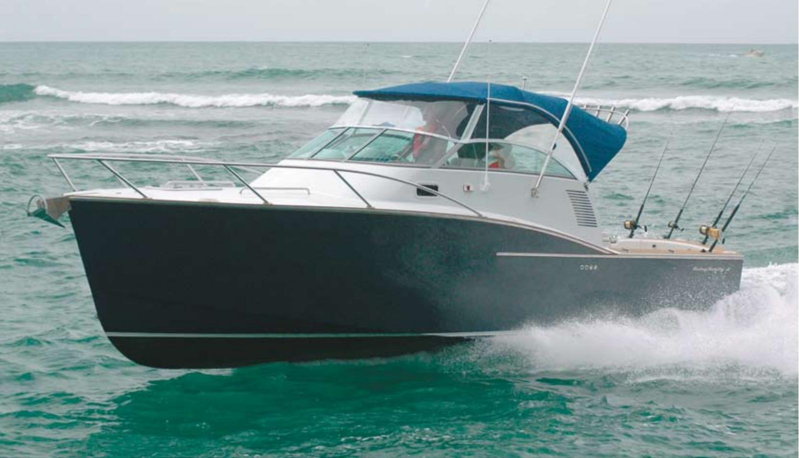
knots; cruising at 2700rpm at 20 knots; top speed 3800rpm at 34 knots. Fuel capacity is 380 litres, giving a range of 300nm at 20 knots.
