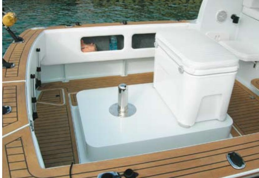
The area under the bridge is fitted with a double berth. Building the rear deck out over the stern leg allows a full walk-around cockpit.
