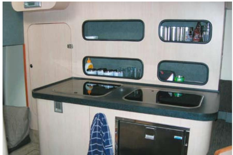
*The galley unit offers a hot and cold freshwater sink, gas cooker, fridge, and plenty of stowage.*
