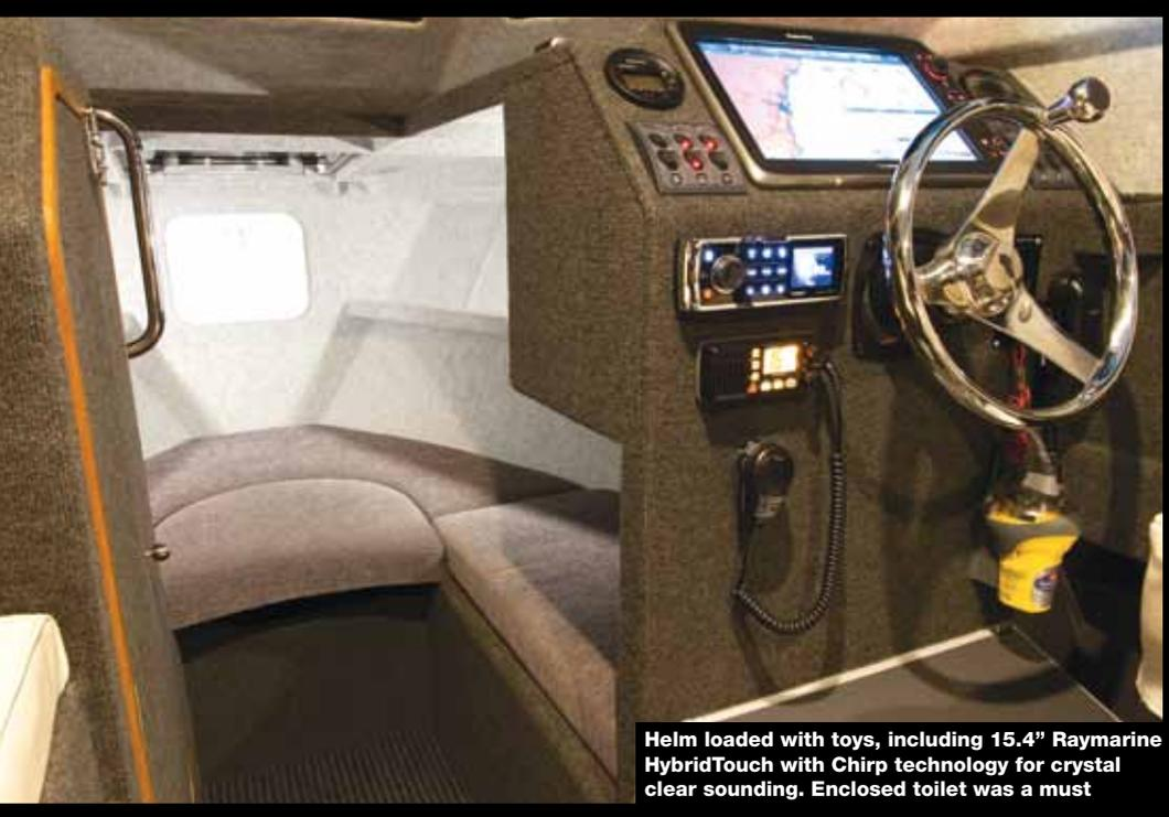
**Helm loaded with toys, including 15.4" Raymarine HybridTouch with Chirp technology for crystal clear sounding. Enclosed toilet was a must**
